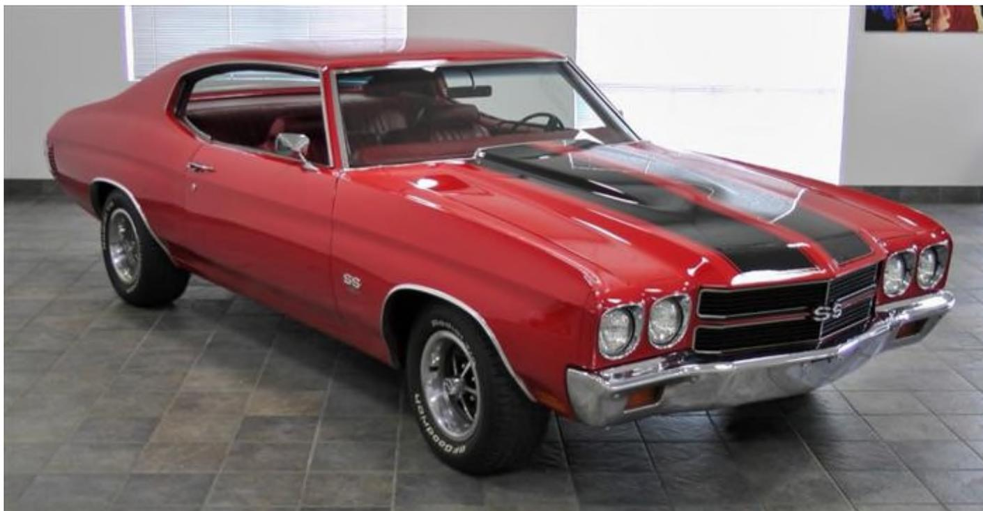
The elegant 454 LS6 are the rarest Chevelles found. In 1970, Chevelle SS came with the option of either getting an RPO225, which had a 402 cubic inch engine, or a RPO215, which had a 440 cubic inch engine. The LS6 was an exclusive model which was only available on RPO215s with an added horsepower of 100, which totaled up to an impressive 560 horsepower.
